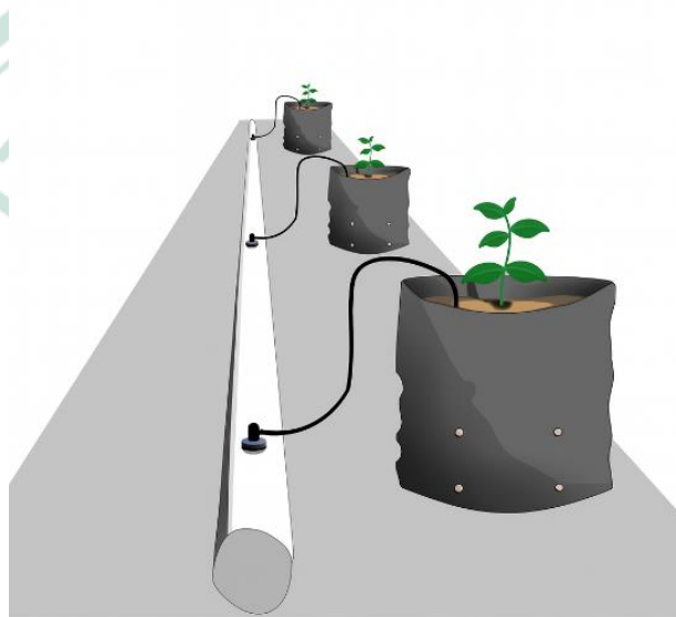
Gambar 2. 2 Sistem Hidroponik Drip Non-Recovery
